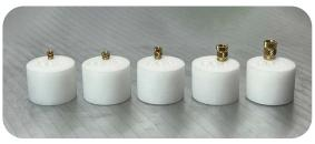
The above shows PA12 Nylon, PETg, PLA, TPU and Onyx test specimens.
